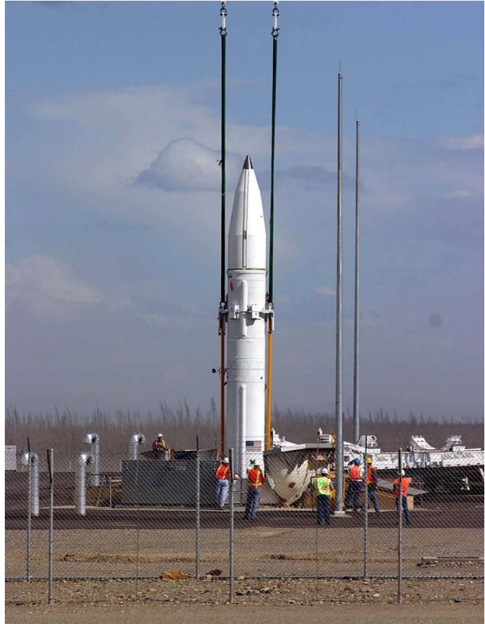
Missile interceptor is lowered into its missile silo at Fort Greely, Alaska (photo: US Army-some rights reserved)
