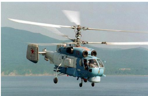
Photo Credit: US Navy, Ka-27 Anti-Submarine Warfare Helicopter
